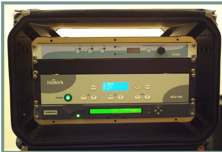
The Transmit case contains the HPA controller, ACU100 and the DVB-S Satellite modulator and the video encoder. Other configurations available.
